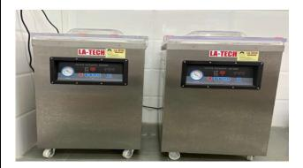
No of Machine: 2 Packing Speed: - 2-3 Minutes Take each round 6 Packet. Description
