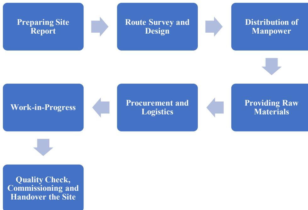
1. **Preparing site report-** Firstly we conduct a comprehensive survey of the railway tracks to assess the terrain, existing infrastructure, and any potential obstacles or challenges and also identify suitable locations for laying the optical fiber cable, considering factors such as accessibility, proximity to existing utility lines, and minimizing disruption to railway operations.
